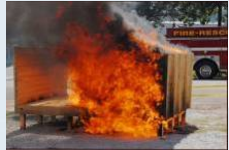
TimberSIL ® (left side) not burning; composite decking and vinyl siding engulfed (right side)
