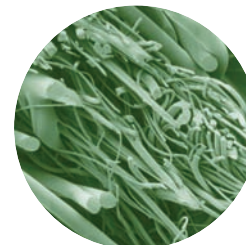
RoofShield triple layer spun bond polypropylene
